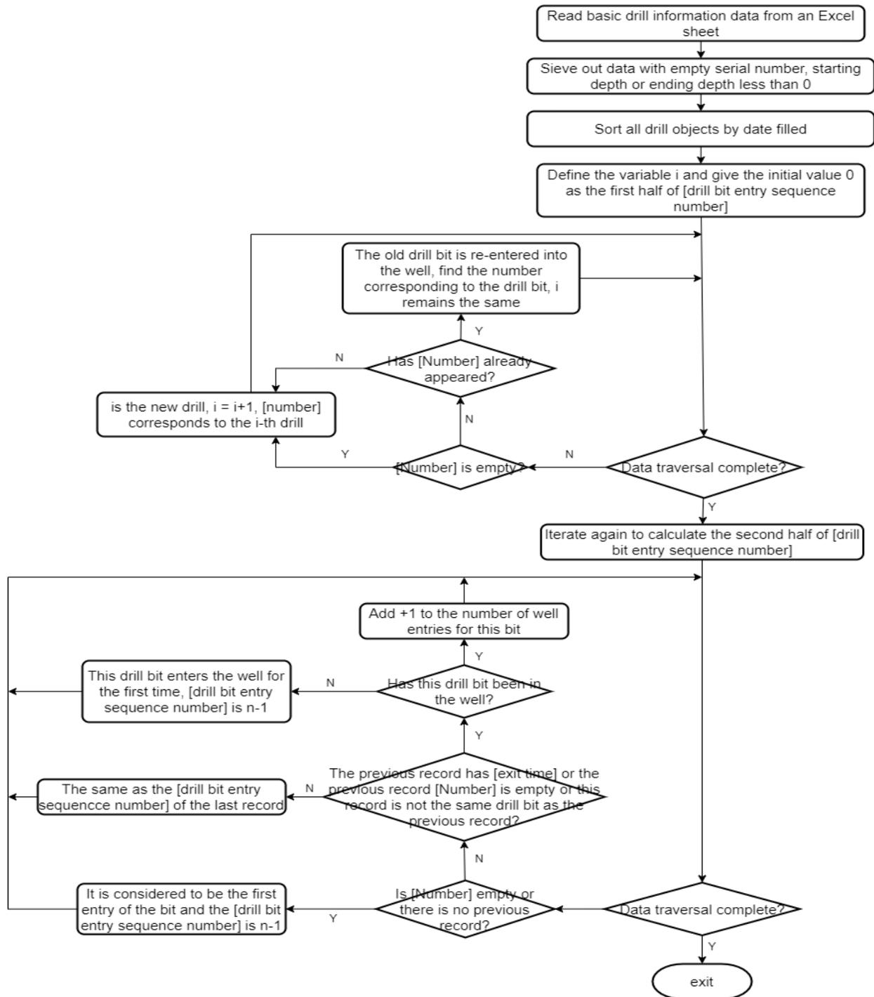
Figure 1. Flowchart for generating the drill bit entry sequence number
