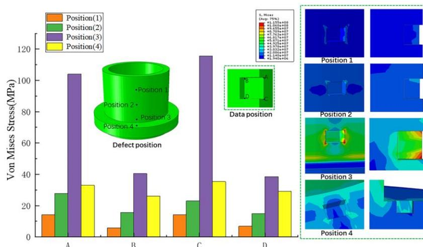
Fig. 5 The stress distribution with different defect positions
