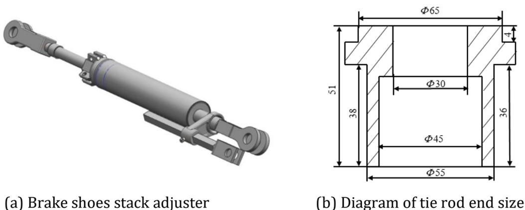
Fig. 1 Dimensions of the parts
