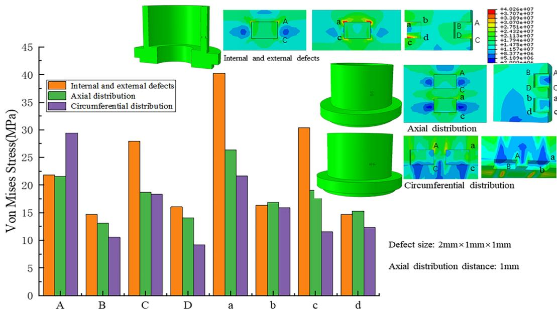
Fig. 6 The stress distribution with double defects
