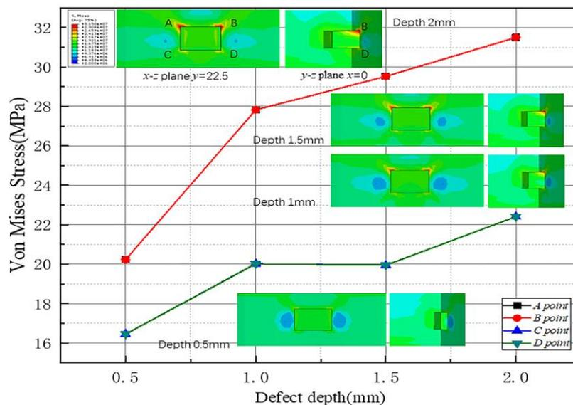
Fig. 3 The stress distribution with different defect depths
