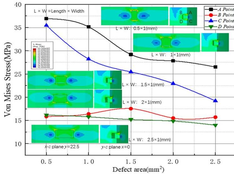
Fig. 4 The stress distribution with different defect areas
