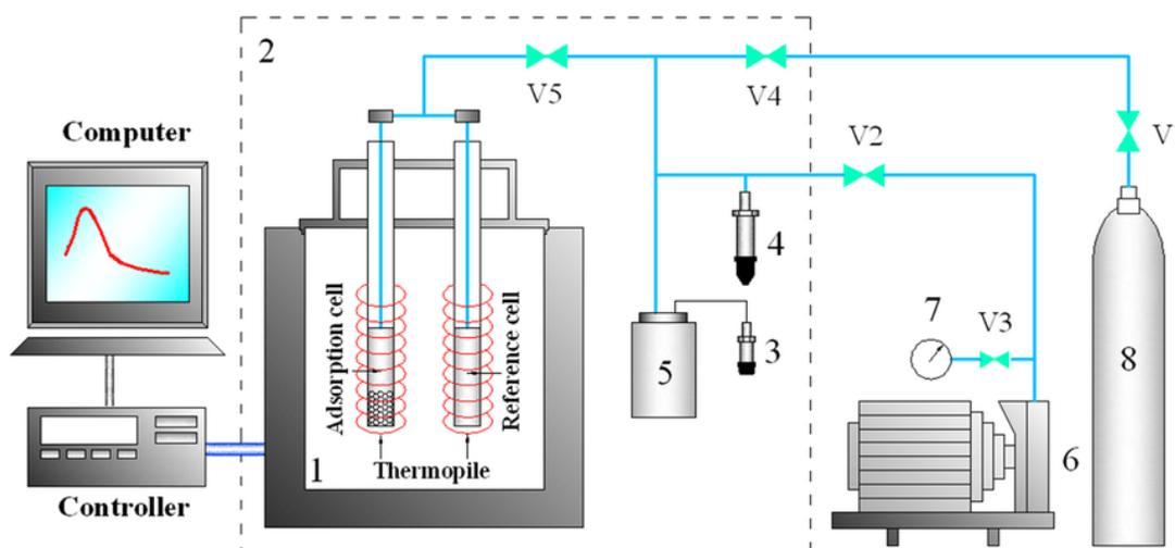
Figure 1. Microcalorimeter C80 test system
