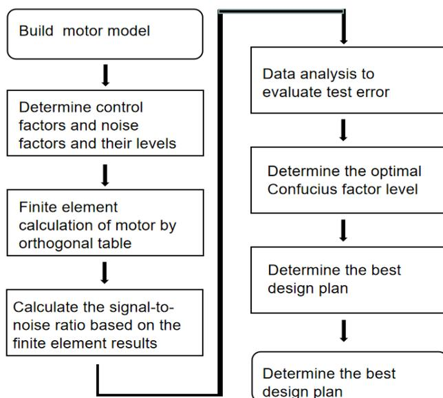
Figure 1. Improved Taguchi Robust Design Process
