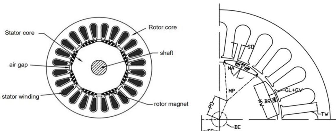
Figure 2. Permanent magnet synchronous motor structure diagram and controllable factor parameter diagram
