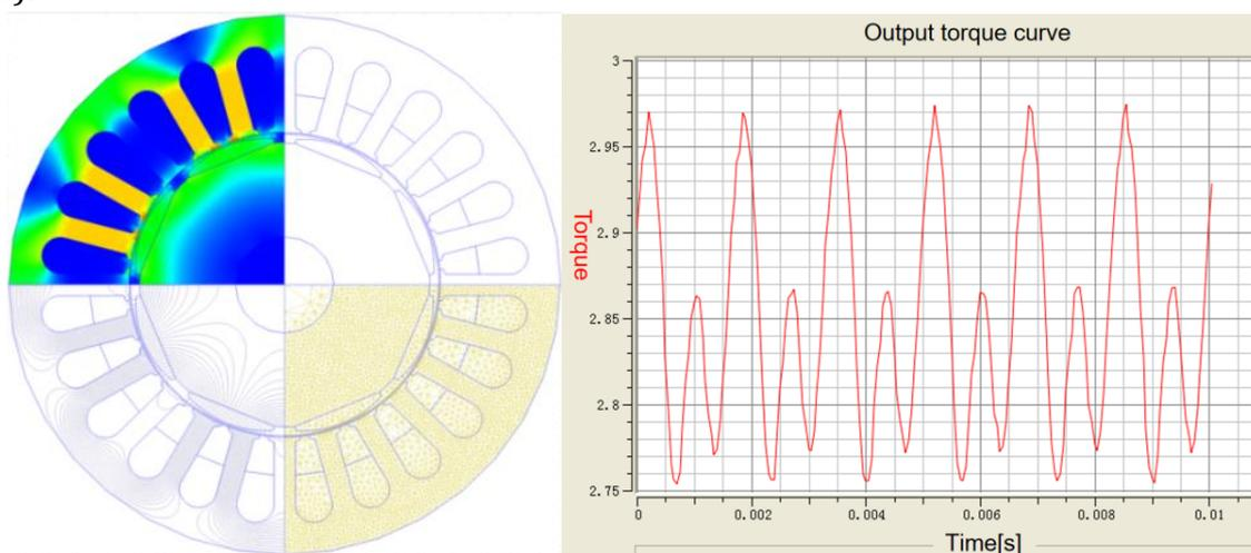
Figure 3. (Left) Motor geometry model, finite element mesh, magnetic field lines and field calculation results (Right) Output torque curve
