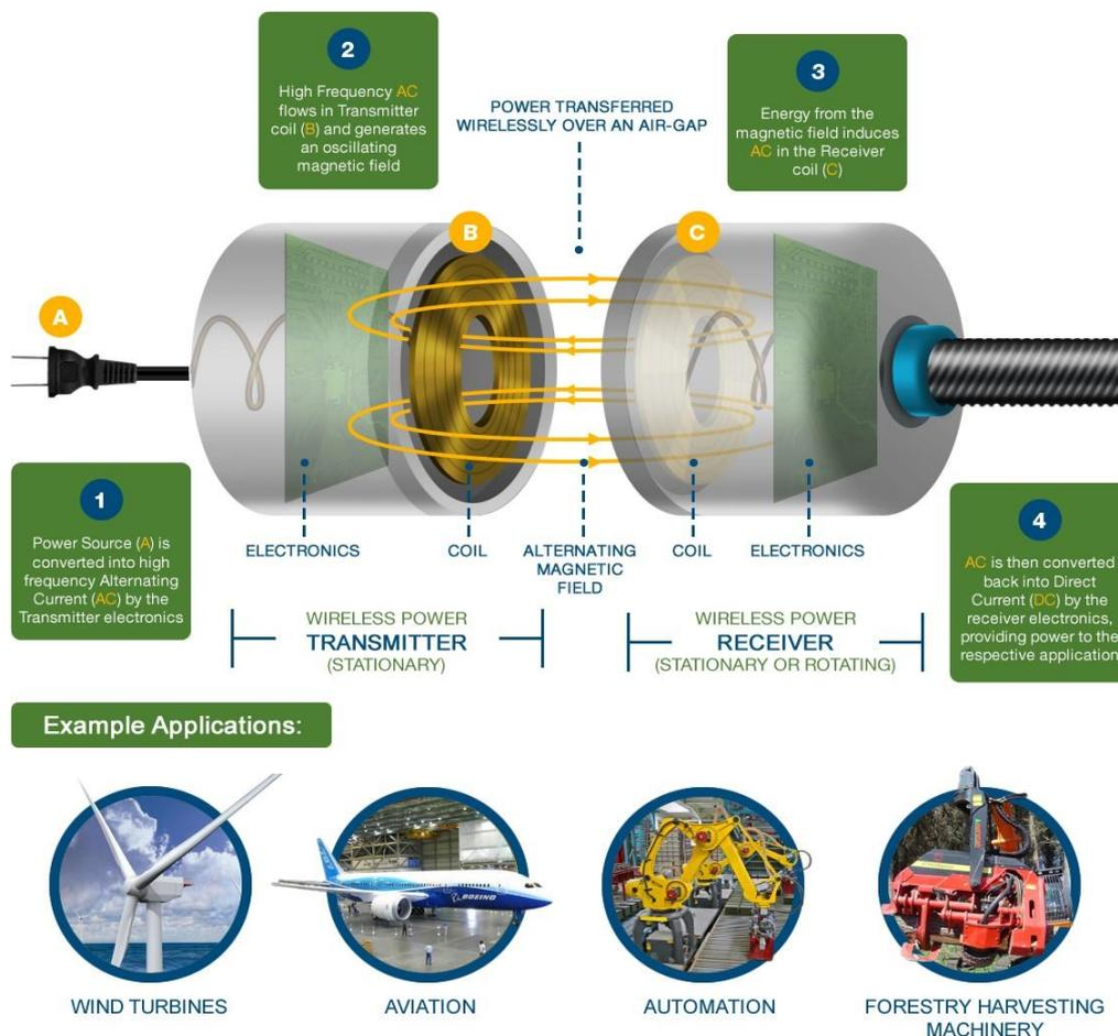
Fig. 2 Illustration for WPT system and its various applications
