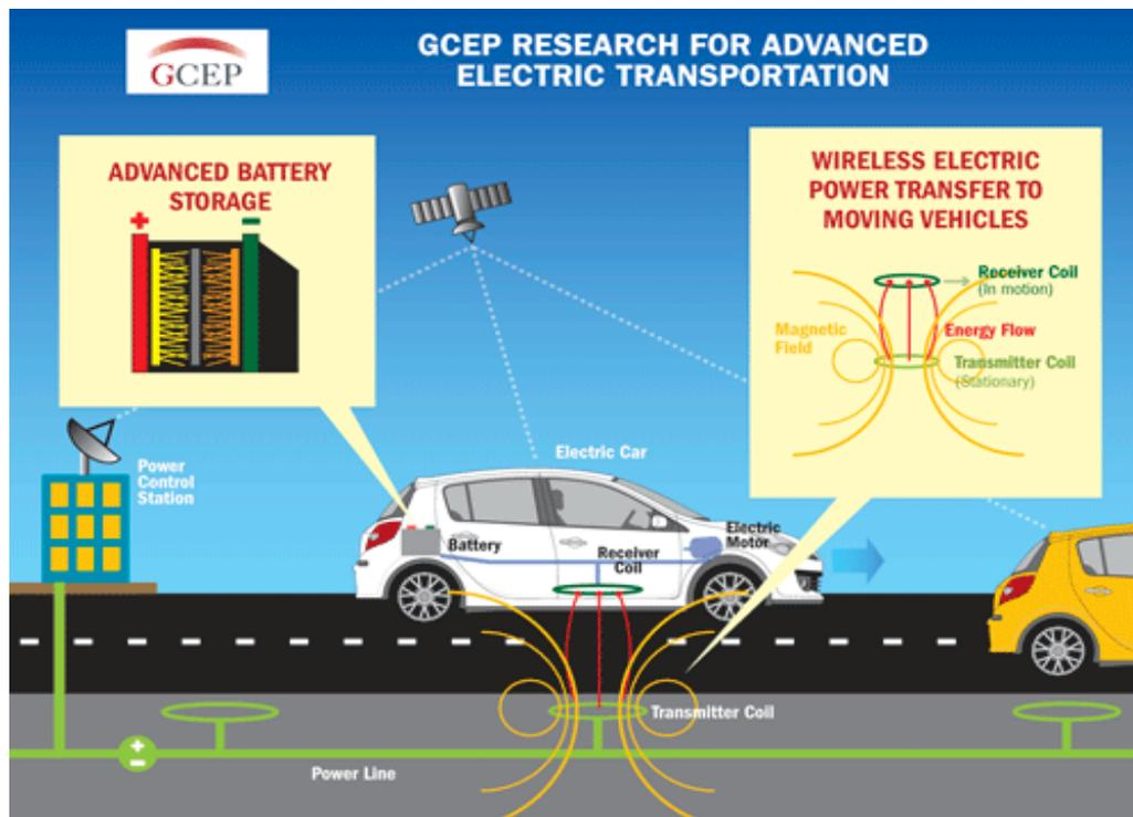
Fig. 1 Illustration of wireless electric power transfer to moving vehicle
