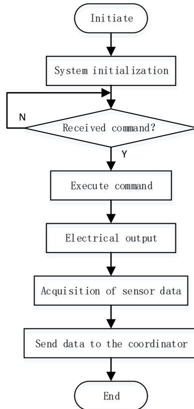
Figure 3. Color lamp controller software flow
