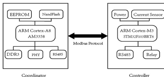
Figure 2. Hardware structure of the system
