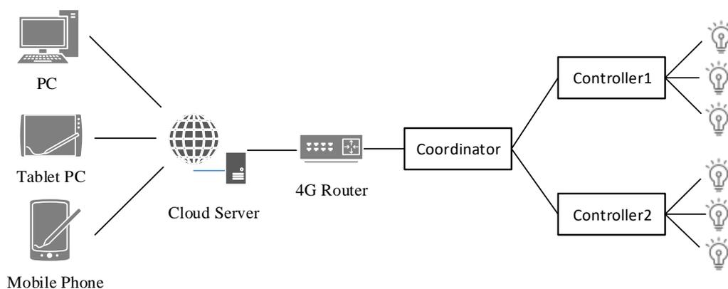
Figure 1. The overall structure of the intelligent lantern control system
