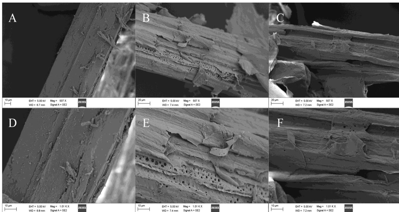
Figure 5. SEM images of raw SCB (A, D), the SCB pretreated by pretreatment T1 to obtain the highest TFSC (B, E), and the SCB pretreated by pretreatment T2 to achieve the highest TFSY (C, F) in two magnifications of 507 and 1010, respectively.
