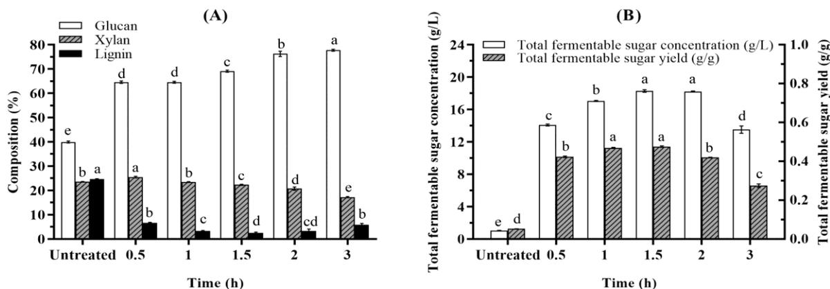
Figure 3. The main compositions (A) and enzymatic saccharification (B) analyses of SCB samples pretreated with 7% Na<sub>2</sub>CO<sub>3</sub> in 20% aqueous ammonia for different time at 220 °C. The same letter suggests no significant difference ( $p > 0.05$ ) at various time among the same composition, TFSY, or TFSC of SCB samples ( $n = 2$ ), respectively.
