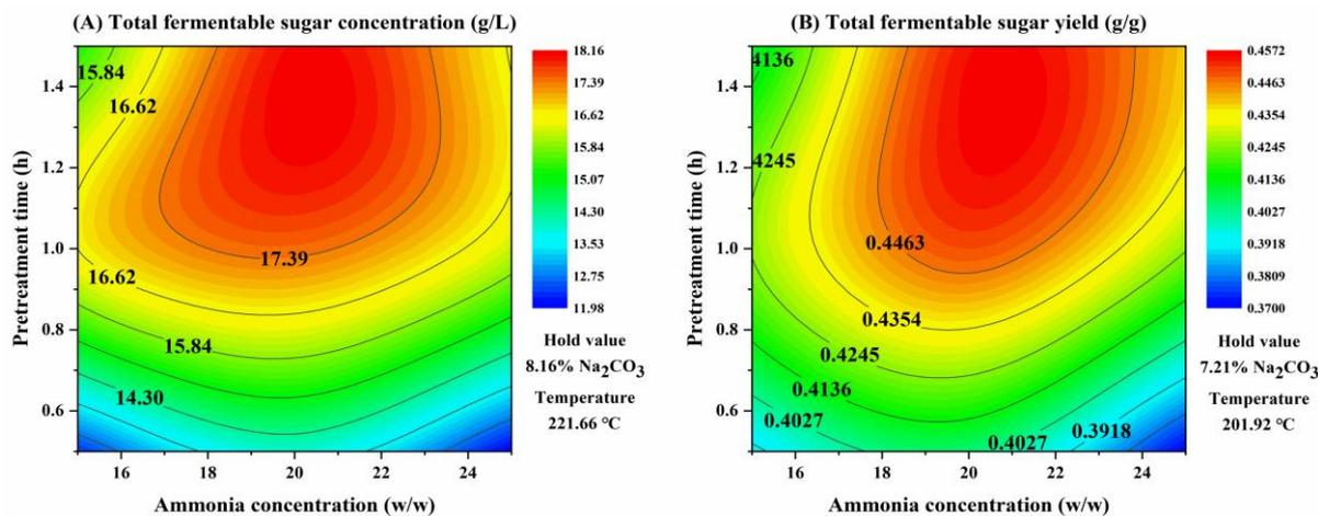
Figure 4. Contour charts revealing the effects of ammonia concentrations and pretreatment time on (A) TFSC with the hold values of 8.16% Na<sub>2</sub>CO<sub>3</sub> and 221.66 °C (optimal conditions were pretreatment time of 1.39 h and ammonia concentration of 20.44%) and (B) TFSY with the hold values of 7.21% Na<sub>2</sub>CO<sub>3</sub> and 201.92 °C (optimal conditions were pretreatment time of 1.38 h and ammonia concentration of 20.42%).
