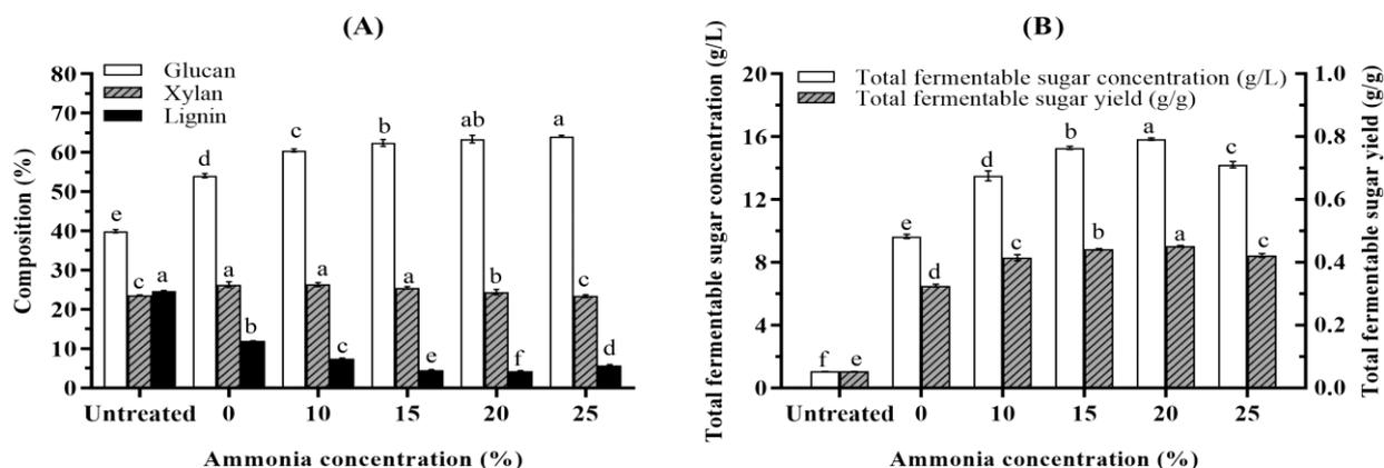
Figure 1. The main compositions (A) and enzymatic saccharification (B) analyses of SCB samples pretreated with different concentrations of aqueous ammonia containing 7%  $\text{Na}_2\text{CO}_3$  at 200 °C for 1 h. The same letter suggests no significant difference ( $p > 0.05$ ) at various concentrations of aqueous ammonia among the same composition, TFSY, or TFSC of SCB samples ( $n = 2$ ), respectively.
