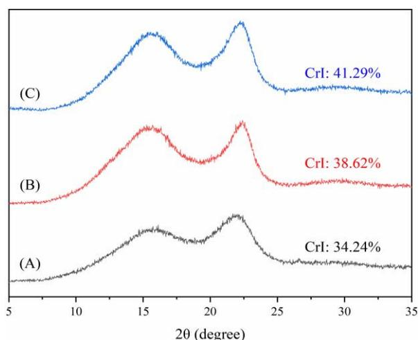
Figure 7. XRD patterns and corresponding CrI of raw SCB (A), the SCB pretreated by pretreatment T1 to obtain the highest TFSC (B), and the SCB pretreated by pretreatment T2 to achieve the highest TFSY (C).
