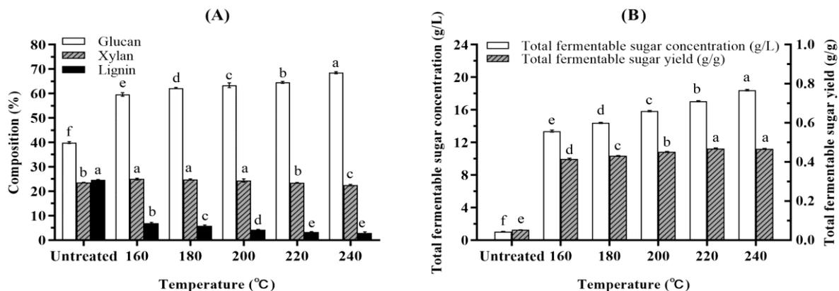
Figure 2. The main compositions (A) and enzymatic saccharification (B) analyses of SCB samples pretreated with 7% Na<sub>2</sub>CO<sub>3</sub> in 20% aqueous ammonia at different temperatures for 1 h. The same letter suggests no significant difference ( $p > 0.05$ ) at various temperatures among the same composition, TFSY, or TFSC of SCB samples ( $n = 2$ ), respectively.
