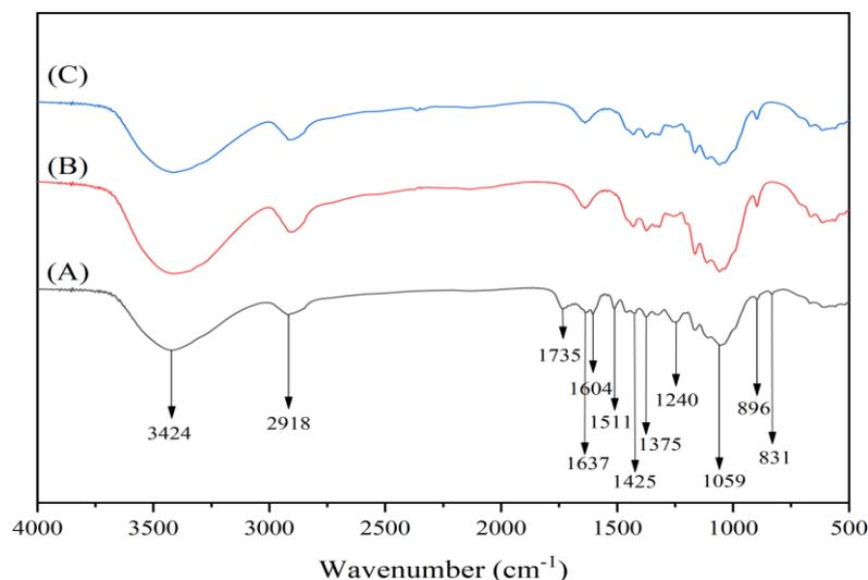
Figure 6. FTIR spectra of raw SCB (A), the SCB pretreated by pretreatment T1 to obtain the highest TFSC (B), and the SCB pretreated by pretreatment T2 to achieve the highest TFSY (C).
