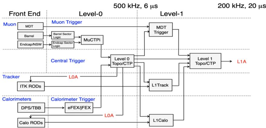
Figure 3. A block diagram of the architecture of the Split Level-0/Level-1 hardware trigger proposed for the Phase-II upgrade. (The MDT trigger is shown as part of Level-1 but may be used at Level-0).[4]
