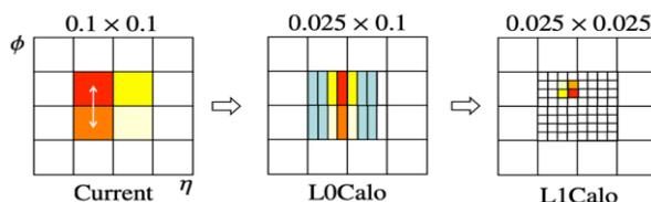
Figure 4. The EM granularity available in the current Phase-II Level-0 and Phase-II Level-1 EM triggers.[4]
