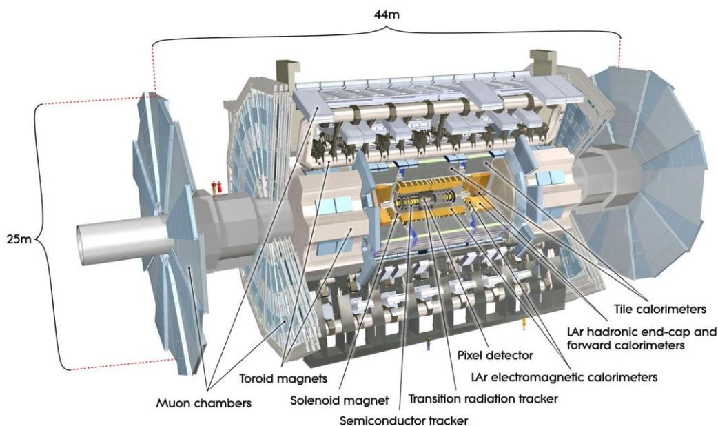
Figure 2. The structure of the ATLAS Detector[3]
