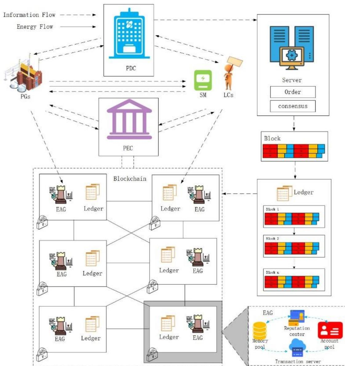
Figure 1. The system of direct power purchase by LCs under the consortium blockchain framework
