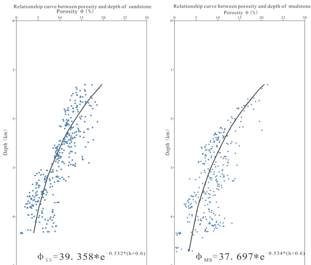
Figure 2. Relation curve between porosity and depth of sandstone and mudstone of Study Area
